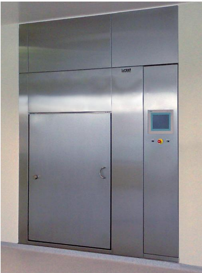
Depyrogeneration oven loading side with semi-automatic door
